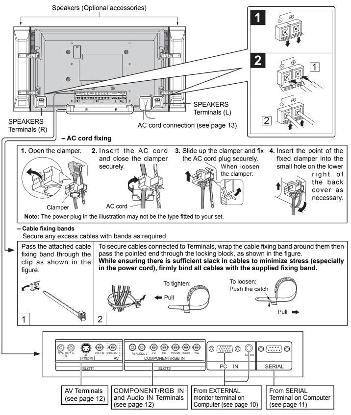
Note: At factory shipment, Terminal boards are installed in SLOT 1 and SLOT 2.
